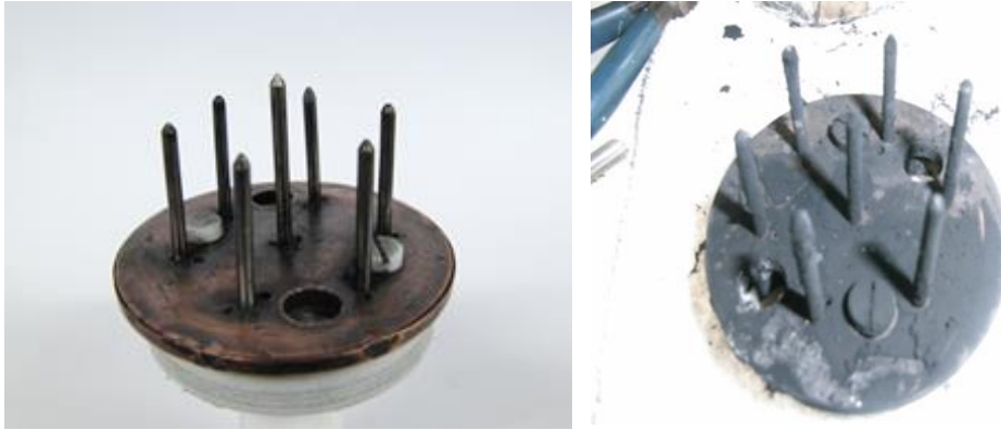
Fig. 5 Condition of antennas/electrodes before and after methane hydrate decomposition.
