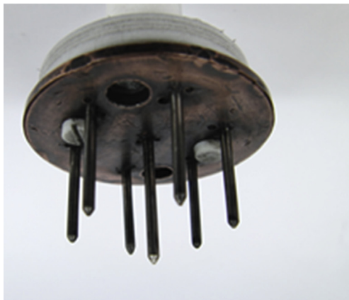
Fig. 6. Condition of antennas/electrodes before and after methane hydrate decomposition.
