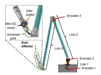
Figure 4. Haptic device and its components.
