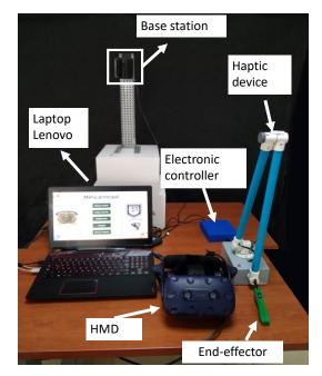
Figure 5. Components of the rehabilitation system.
