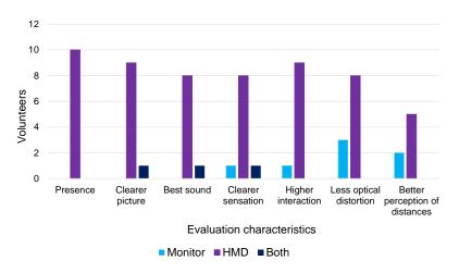
Figure 10. Characteristics of the system according to the display system (monitor or HMD).
