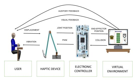
Figure 1. The architecture of the UL Rehabilitation System.
