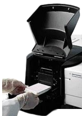
Figure 19. A) Cary Eclipse Fluorescence Spectrophotometer. B) Microplate reader accessory.
