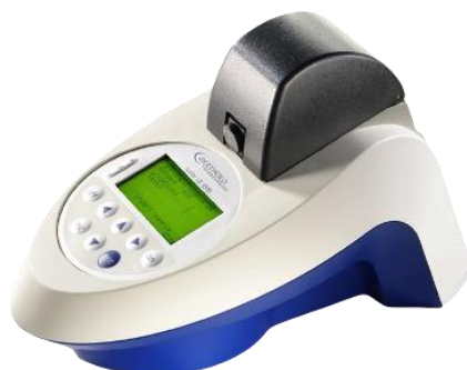
Figure 18. Portable tube luminometer from Berthold Technologies.
