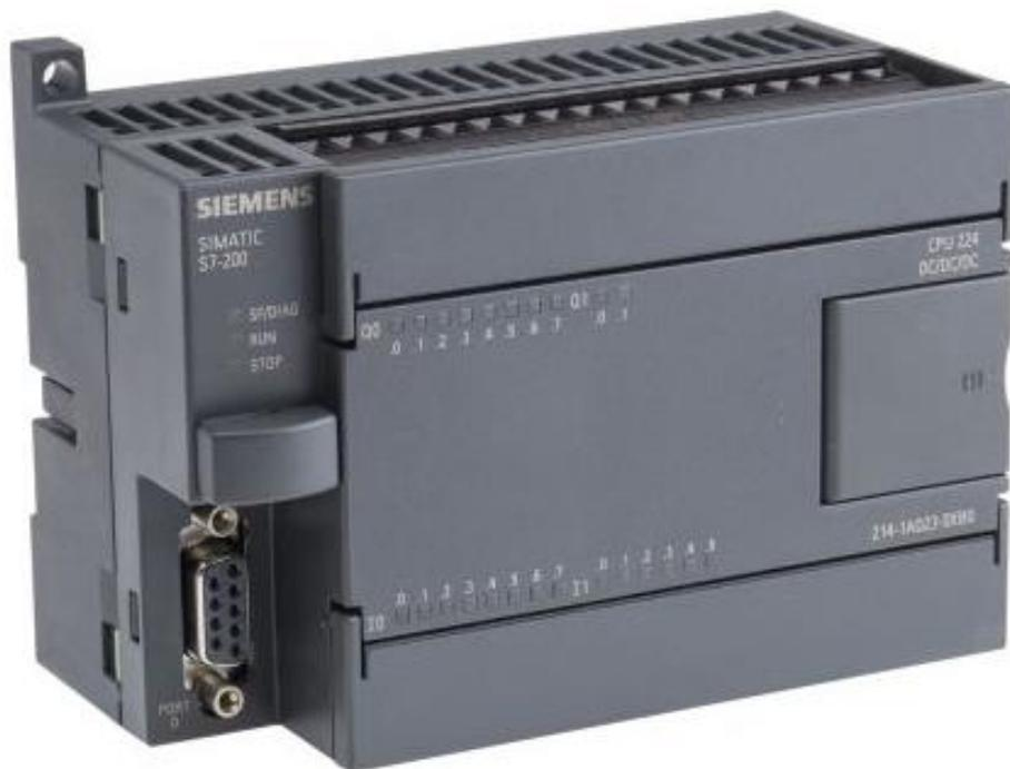
**Figura III.5:** PLC S7-200 CPU 224.
