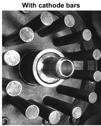
Fig. 3. Electrode configuration with cathode bars. The anode A3 is used in this configuration.
