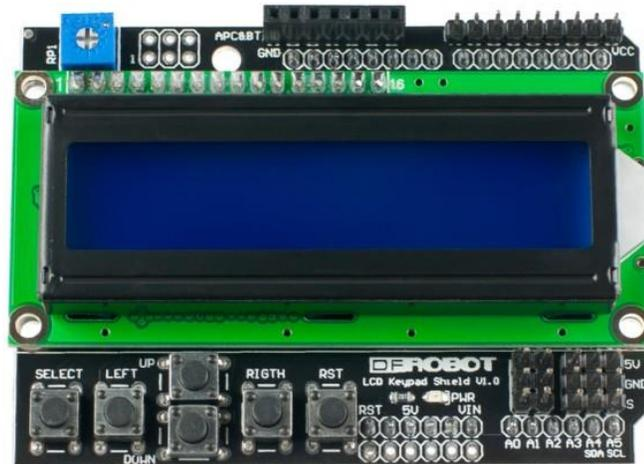
Figura 1.9: Pantalla LCD KeypadShield
