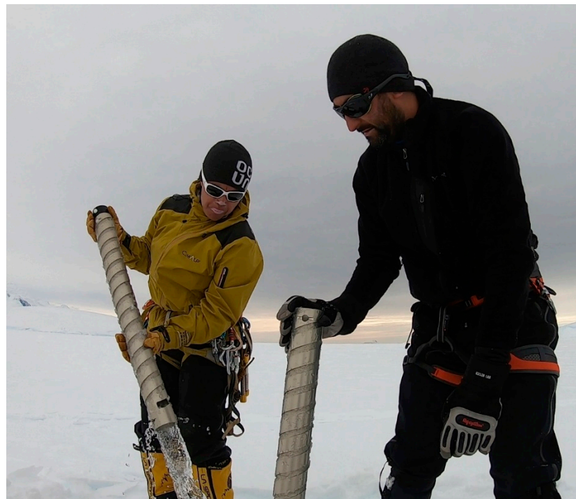
Figure 4. Water being drained from the upper section of the drill after the extraction of the lower section of M3. In Video S1, a video of the extraction of the lower section of core is included.
