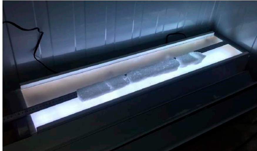
Figure 3. Photograph of the constructed light box. The displayed core is approximately 90 cm in length.
