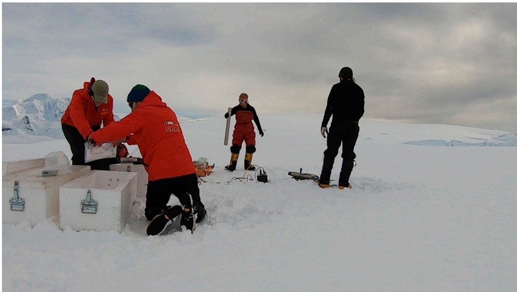
Figure 2. Photograph of core handling on the Müller Ice Shelf. Two team members operated the electric drill, whilst the other two members bagged and recorded the extracted cores.
