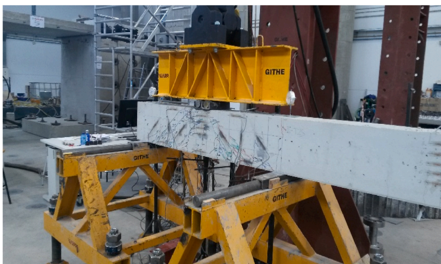
Fig. 3. Lay-out of the shear test.
