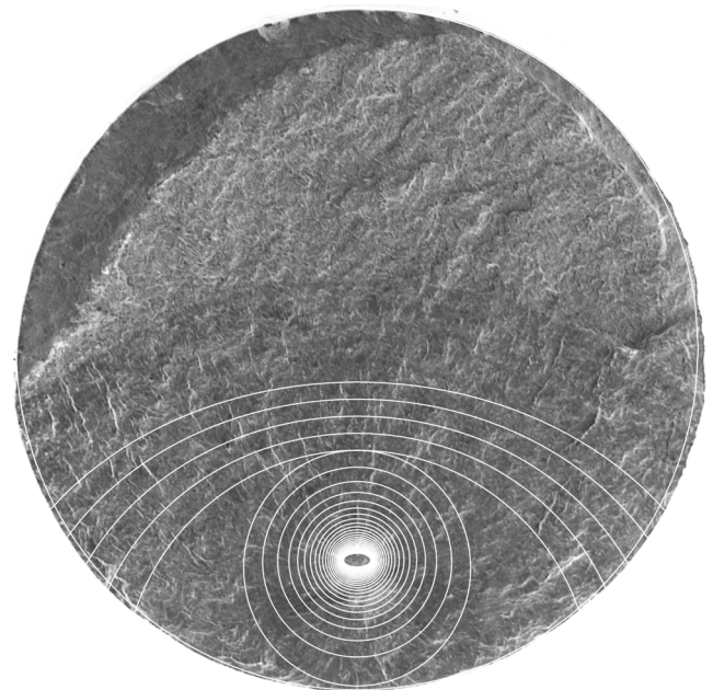
Fig. 11. Fatigue crack growth propagation with recategorization from an embedded crack to a surface crack (fractography courtesy of Niendorf [5]).
