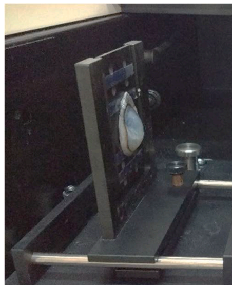
Fig. 1. Bovine cornea placed in the solid sample holder of the Agilent Cary 60 UV–vis spectrophotometer.
