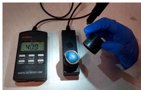
Fig. 2. Bovine cornea placed in the cylindrical holder between the light source and the lux meter.
