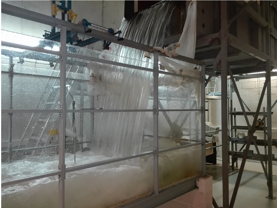
Fig. 2. Detail of the plunge pool in the experimental facility with the optical fiber probe.
