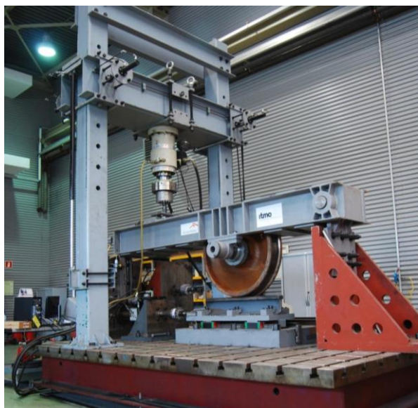
Figure 1. Test rig adapted to perform RCF tests
