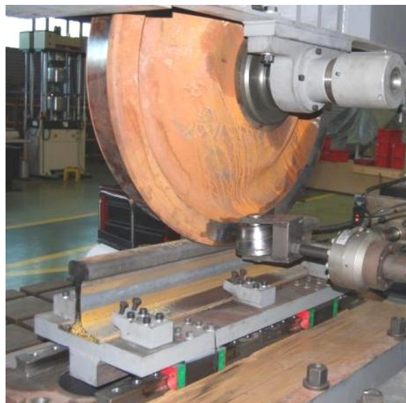
Figure 2. Detail of moving table and lateral load actuator.
