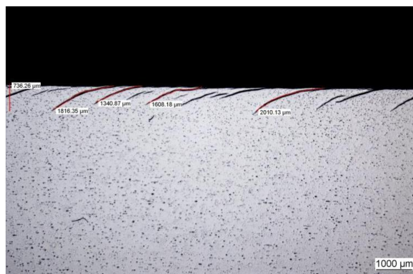
Figure 6. Longitudinal section of the center region of rail n°7 (12.5x). Maximum crack depth: 0.74 mm
