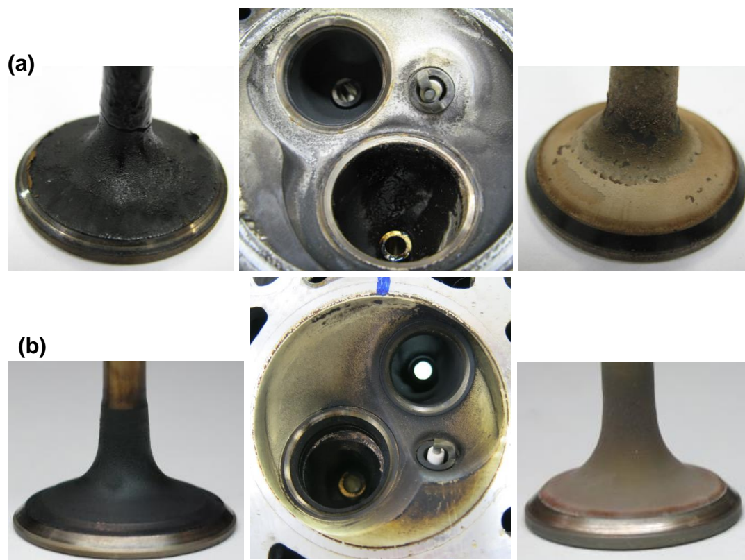
Figure 3. First cylinder with intake and exhaust valves of engine (a) MT-1 (b) MT-2.
