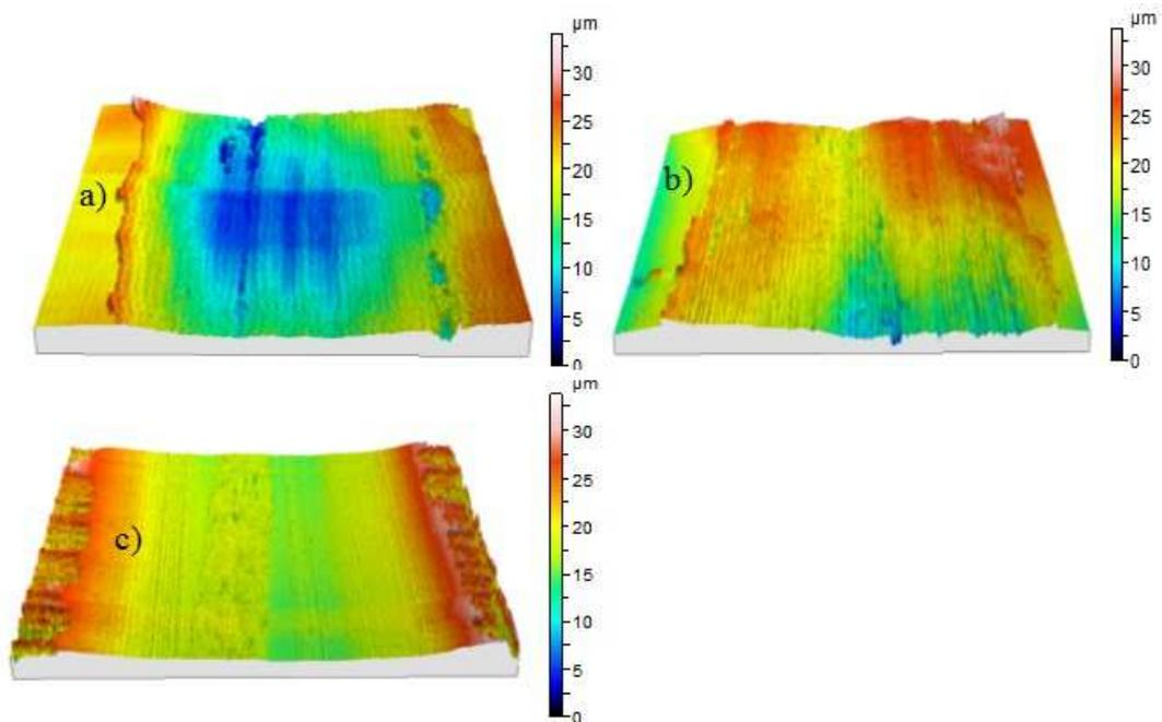
Figure 4. 3D profilometer images of sliding surfaces. a) Samples M1, b) samples M2, c) samples M3 (1 rps, 40 N, 200 m).
