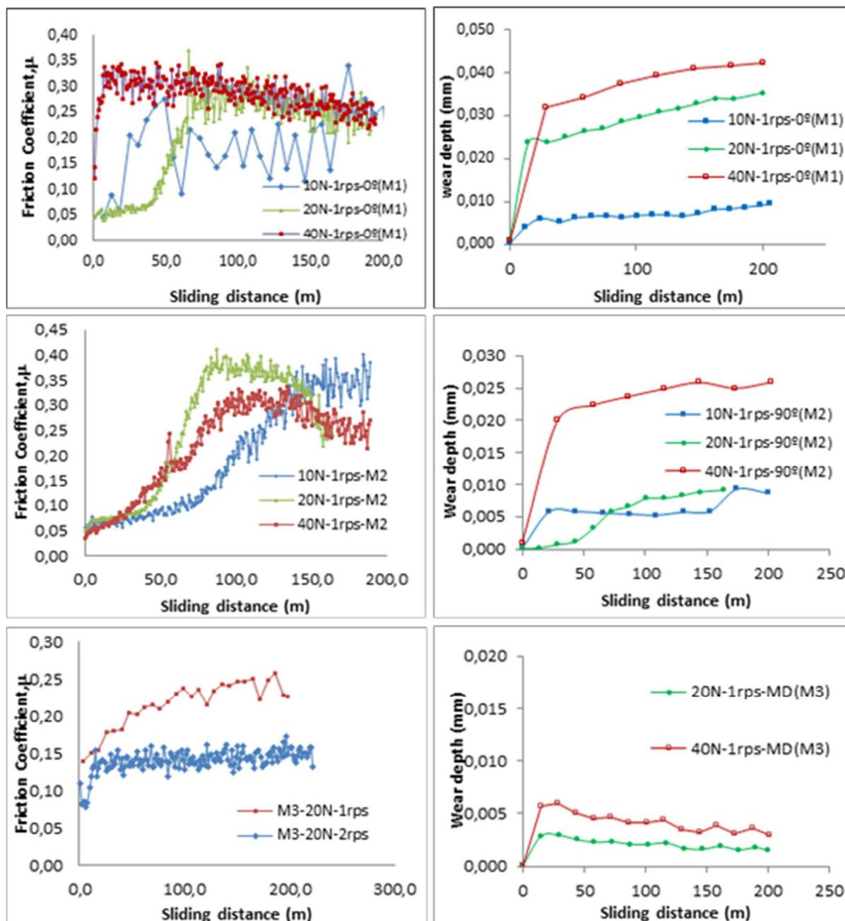
Figure 3 Variation of the friction coefficient and wear depth with sliding distance and load for the three samples of composites experimented.
