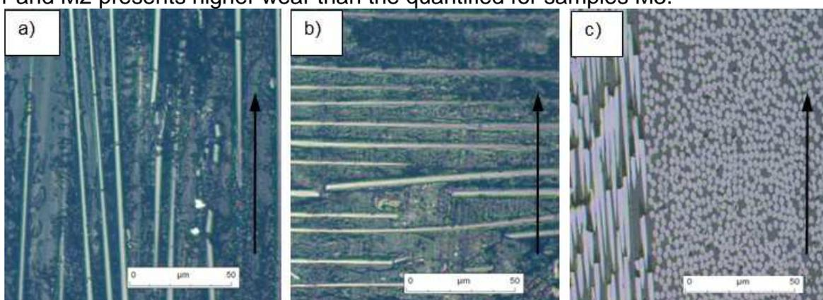
Figure 6. Macrography of the worn surface of samples at 40N and 1rps a) M1, b) M2, c) M3.
