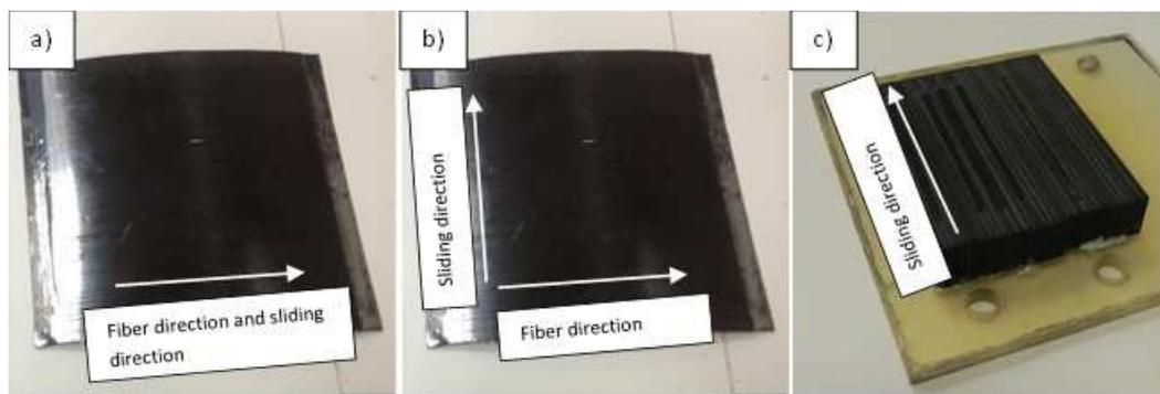
Figure 1. Types of samples configuration; a) Samples M1, b) Samples M2, c) Samples M3.
