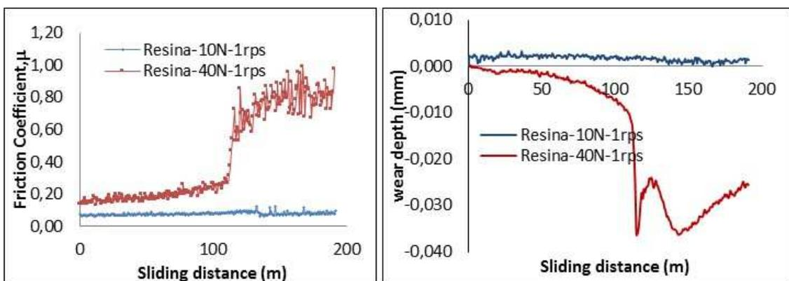
Figure 2. Variation of friction coefficient and wear depth with sliding distance and load for the epoxy resin.
