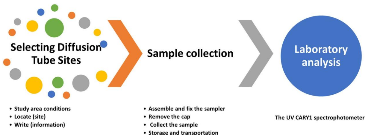
Fig. 3. Diffusive tubes collection and analyzing procedures diagram.
