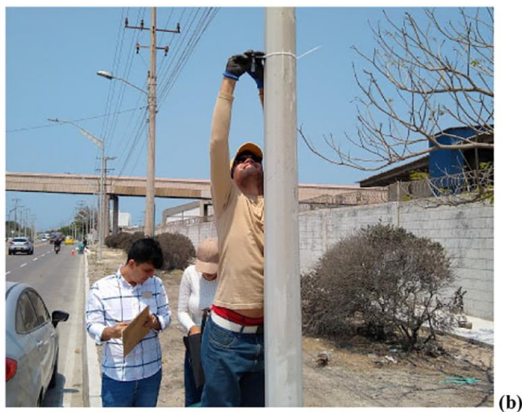
Fig. 2. Diffusion tube for passive sampling of \text{NO}_2 diagram (a) and installation process (b).
