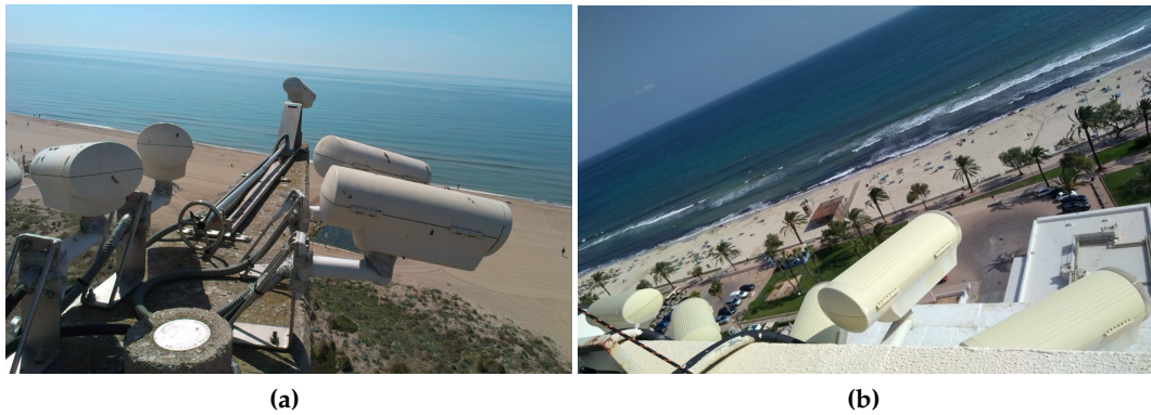
Figure 3.7: Stereo-video coastal observation system at (a) Castelldefels beach and (b) Cala Millor beach.
