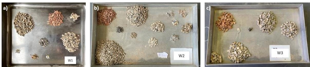
Figure 5. Constituents separation of the three CDW's studied: a) W1; b) W2 and c) W3.
