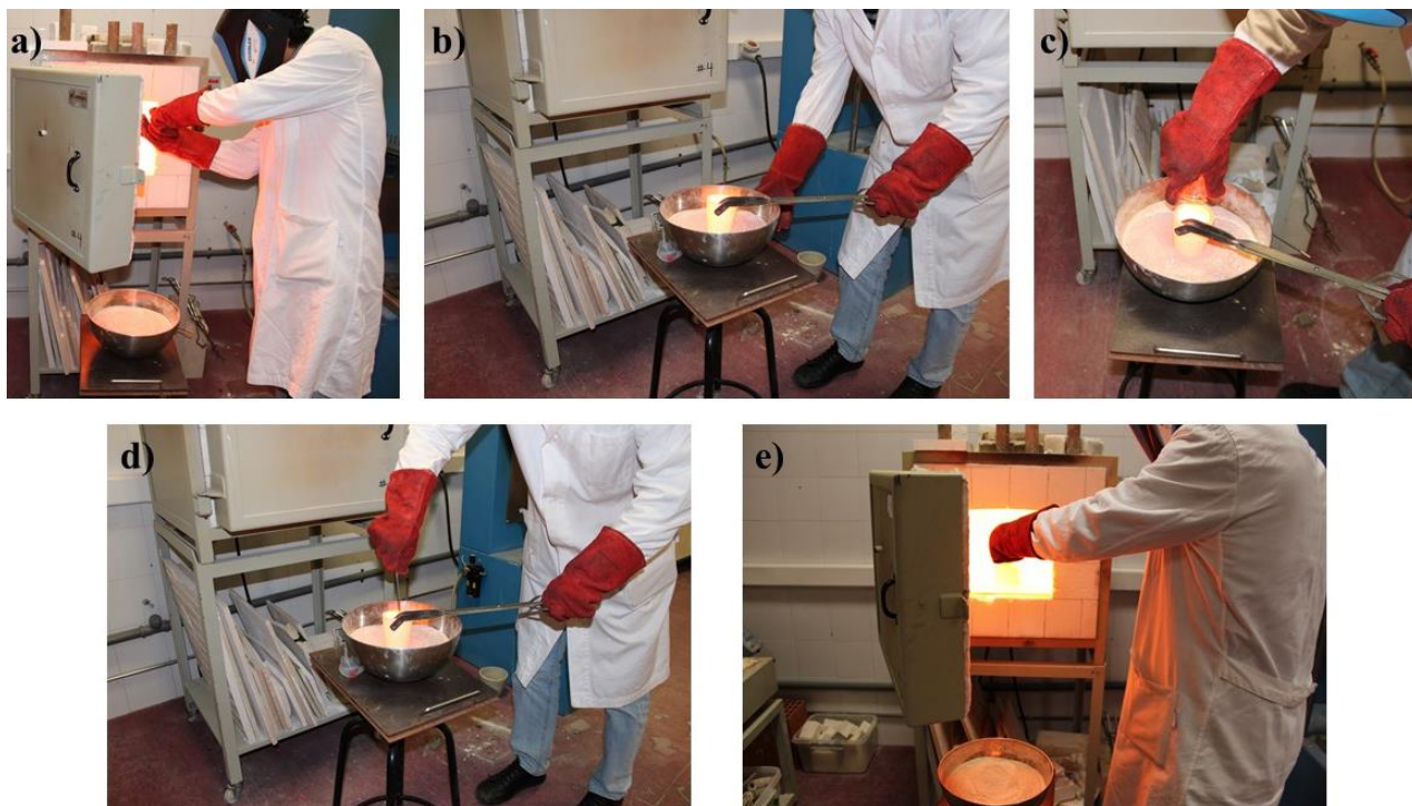
Figure 10.4. Sequence of the definitive procedure: a) the crucible was taken out from the furnace; b) the crucible was deposited on the container with sand; c) addition of the reagents into the molten glass; d) stirring the melt; e) returning the crucible with the molten glass containing the reagents to the furnace.
