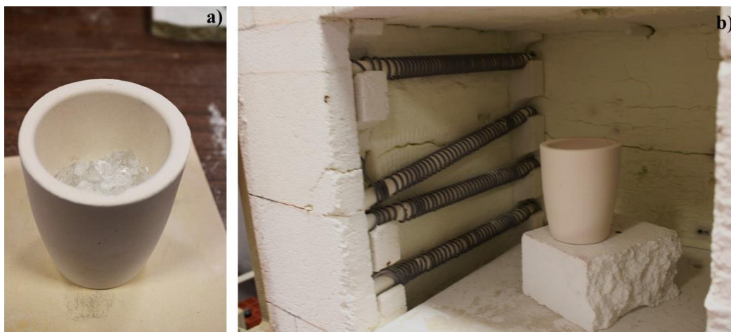
Figure 10.3 a) Crushed glass in the crucible; b) crucible inside the furnace at room temperature.
