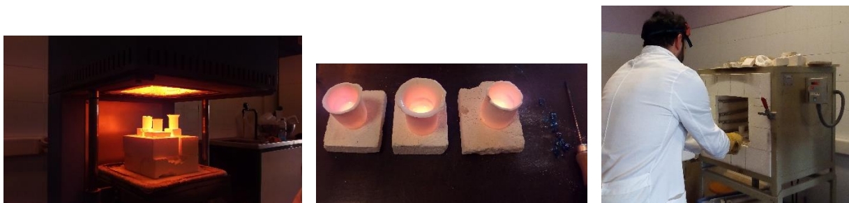
Figure E.1 Sequences of the P1 procedure: a) three batches in the furnace melted at 1300^\circ\text{C} for 3 hours; b) the three crucibles after half hour at 1100^\circ\text{C} and the addition of iron; c) the crucibles were placed in the muffle furnace for the entire night at 550^\circ\text{C} .
