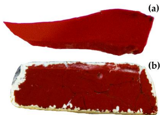
Figure 8.7. Comparison of two fragments of copper red glass: sealing wax (a) and brick red (b).
