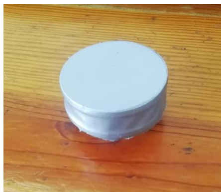
Figure 28 - Float inside the PVC tube
