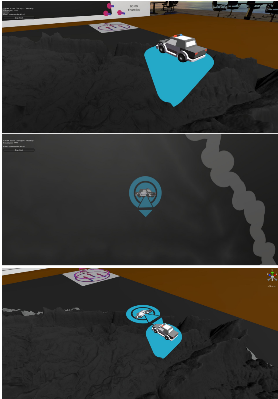
Figure 4.18: Three different close ups of the blue vehicle. Top: 3D Close up. Center: 2D Close up. Bottom: Close up of vehicle in editor, showing both the 3D version and the 2D version, the latter of which is only rendered to the secondary camera.
