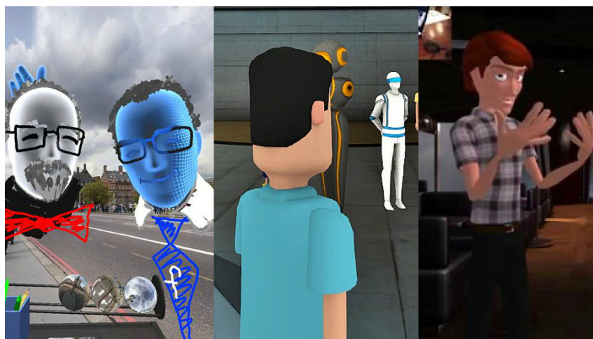
Figure 2.8: Different avatar approaches [17]. Head and hand tracking in Facebook's social VR (left), complete body with predefined animations in AltspaceVR (middle) and complete body with body tracking in High Fidelity (right).
