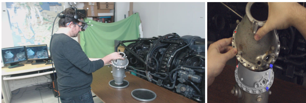
Figure 2.6: Local user with HMD (left). View from local user with virtual replica on display (right) [12].
