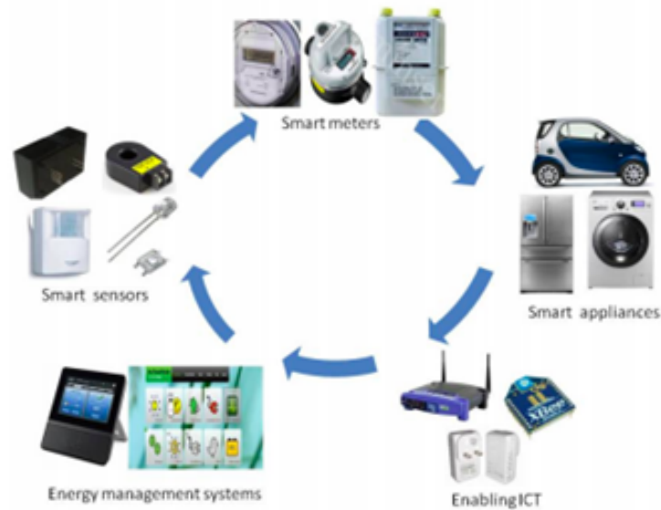
Figure 2: BEMS components (Asare-Bediako et al., 2012)
