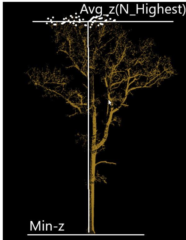
Figure 4.6: Normal Average individual tree height estimation. All N points are given the same weight.
