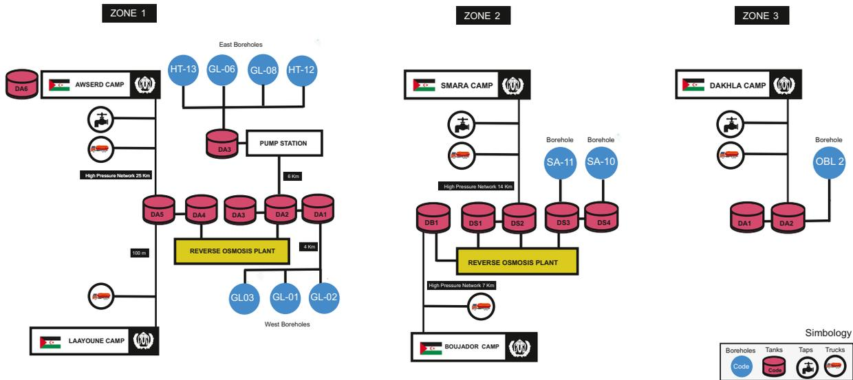
Fig. 2. Sahrawi refugee camps' drinking water supply systems in 2016 in Zone 1 (El Aiun and Awserd), Zone 2 (Smara, Rabouni and Boujador) and Zone 3 (Dakhla) including boreholes (circles), reservoirs (cylinders), reverse osmosis plants and recharge points for tanker trucks.
