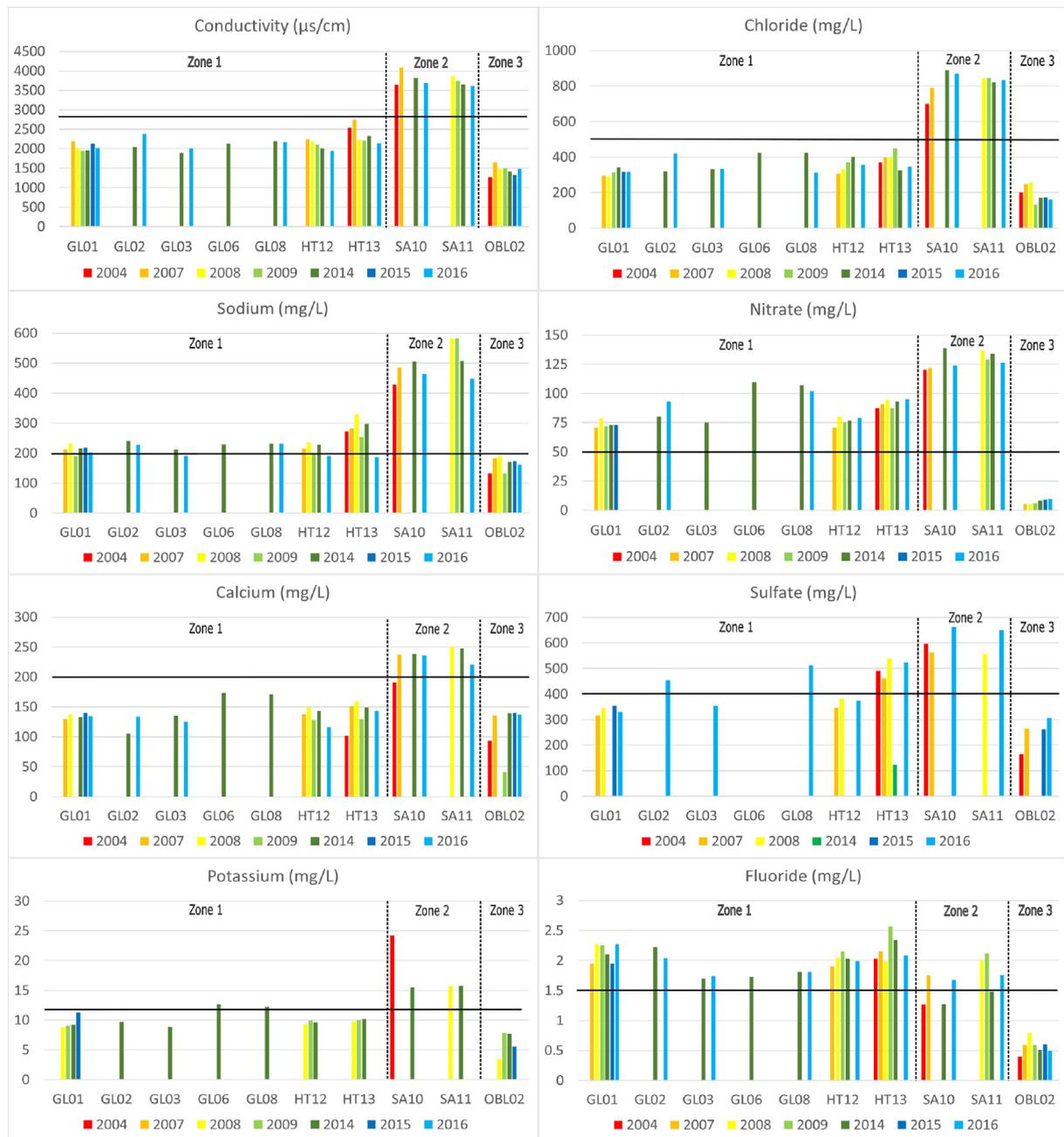
**Fig. 4.** Measured values of chemical parameters on water samples from the pumping wells of the drinking water supply system of the Sahrawi refugee camps from 2004 to 2016 (Table 2 and Table 3). The three zones of the system are distinguished. The parametric value of each parameter according to Algerian regulations (Algeria, 2011) is indicated in each graph by a continuous black line.
