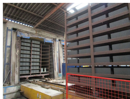
Fig. 15. Curing place for masonry units.
