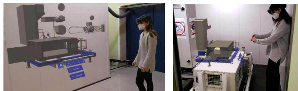
Figure 2. Expanded view of the parts of the digital twin of the cooler (left) and user performing a repair procedure on the real cooler, being guided by the developed AR application (right).
