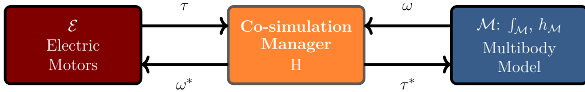
Figure 6.8: Co-simulation diagram of the prototype test bench, arranged following a torque-angular speed coupling scheme.
