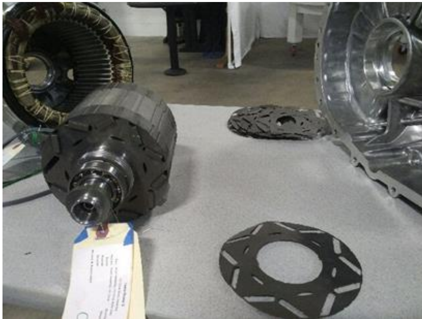
Figure 3.6: A PMSM for automotive applications.
