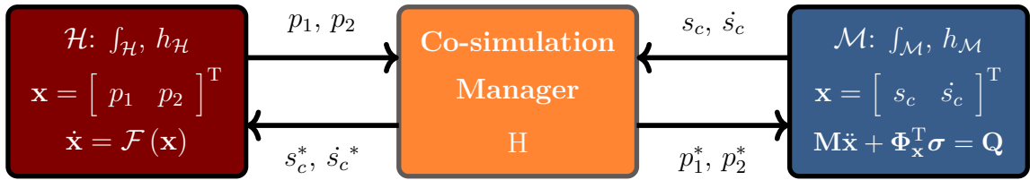
Figure 5.24: The hydraulic crane arranged following a pressure-displacement coupling scheme.
