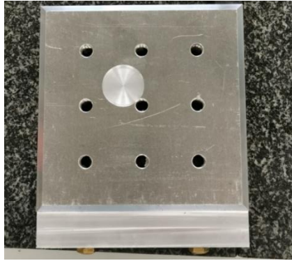
Figure 3. Detail of the inner surface of the Al plates, showing the 9-mm diameter perforations for the AE sensors and the 30-mm recess to protect strain gages.
