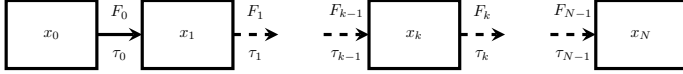
Fig. 1. Dynamic programming problem. At each stage k \in \{0, 1, \dots, N-1\} a control action u_k = F_k x_k is applied during the interarrival time \tau_k .
