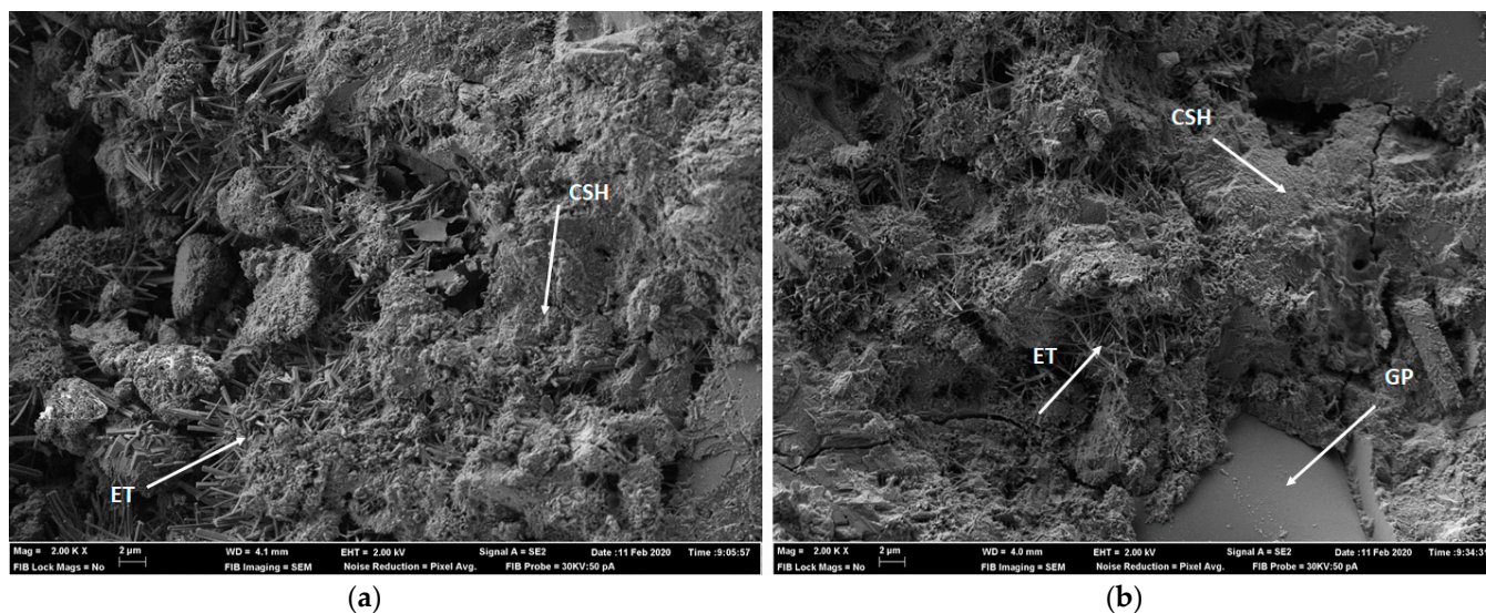
Figure 6. SEM analysis images for the control paste (a) and the GP paste (b) at 2000 \times magnification.
