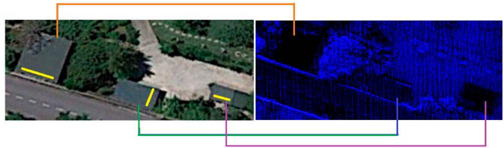
Figure 12. Point cloud on top of three zinc roofs. The yellow lines on top of the roofs represent the orientation of the tiles.
