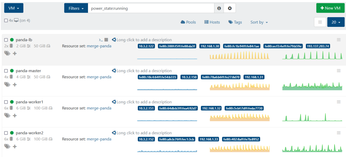
Figure 29 - The 4 hosts forming the cluster – 3 Kubernetes nodes and 1 edge node, all running on Xen Orchestra
