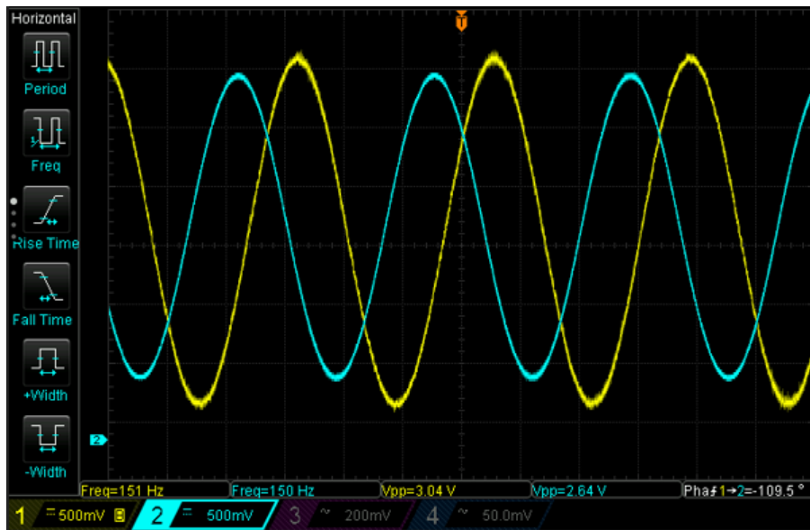
Figure 4.4: Filter input and output signal at 150 Hz.
