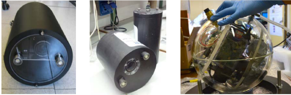
Figure 2.8: Three different enclosures for the GUARD1 system. Left: for deployment on depths up to 40 m. Center: for deployment on depths up to 400 m. Right: for deployment on depths up to 10000 m. [17].
