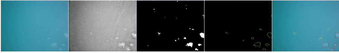
Figure 2.9: GUARD1 image processing steps. From left to right: original image, image enhancement with CLAHE, background/foreground segmentation, contour extraction from original image with Sobel operator, and ROI identification [16].
