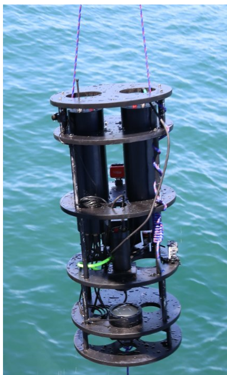
Figure 1.2: MarinEye system with the zooplankton imaging sensor.
