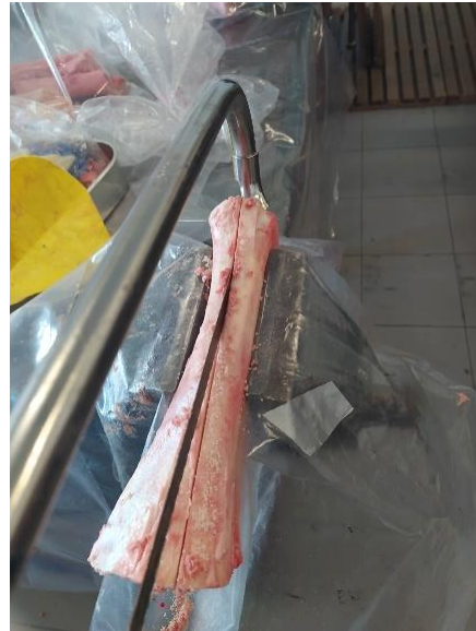
Figure 28 – Step of cutting longitudinally the diaphysis
