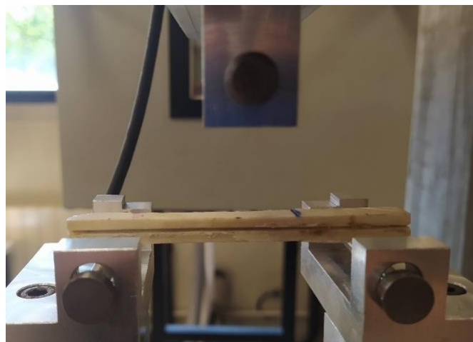
Figure 44 – Setup for the ENF test
