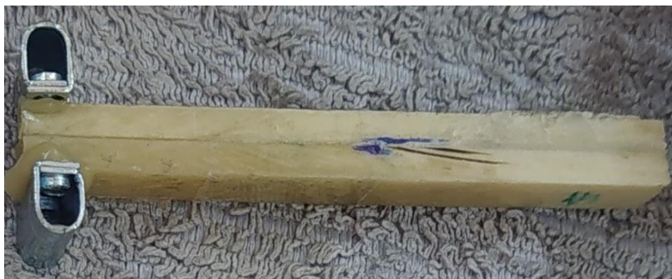
Figure 40 – Specimen for the DCB test
