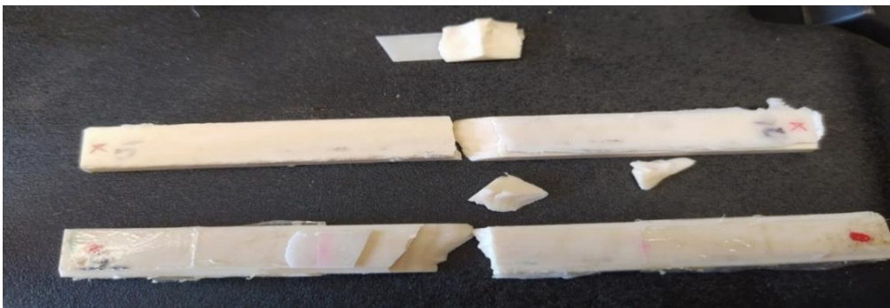
Figure 59 – Specimen 5 fractured after the ENF test
