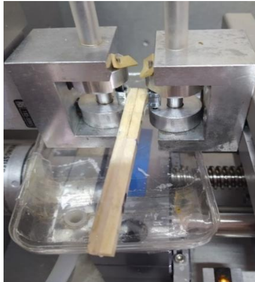
Figure 41 – Setup for the DCB test
