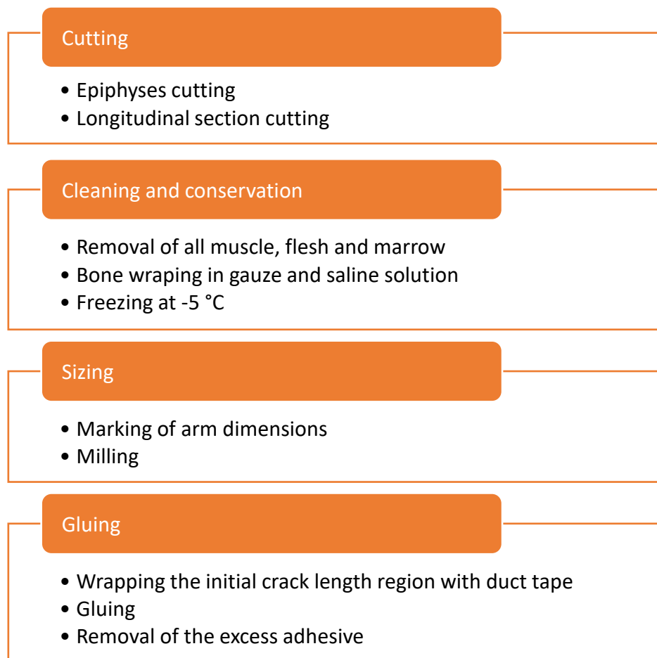
Figure 26 – Stages for the specimen' manufacturing processes
