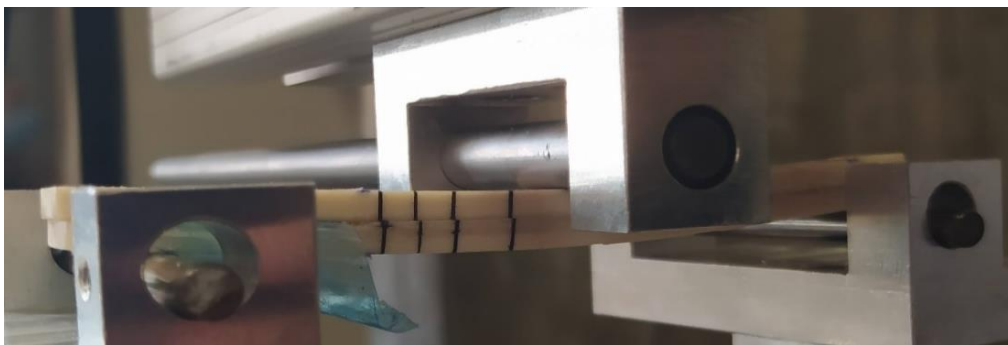
Figure 60 – Loaded specimen in the ENF test
