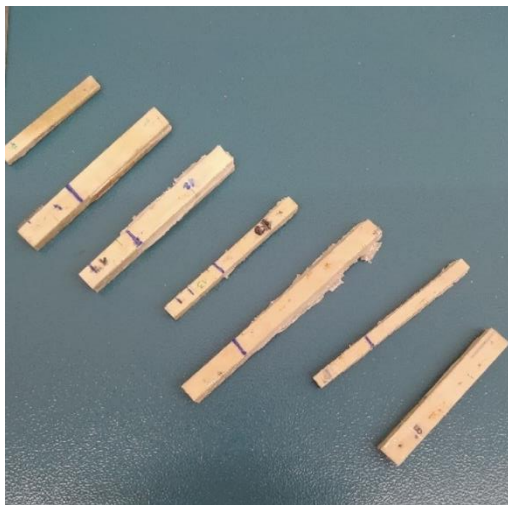
Figure 37 – Specimens after gluing
