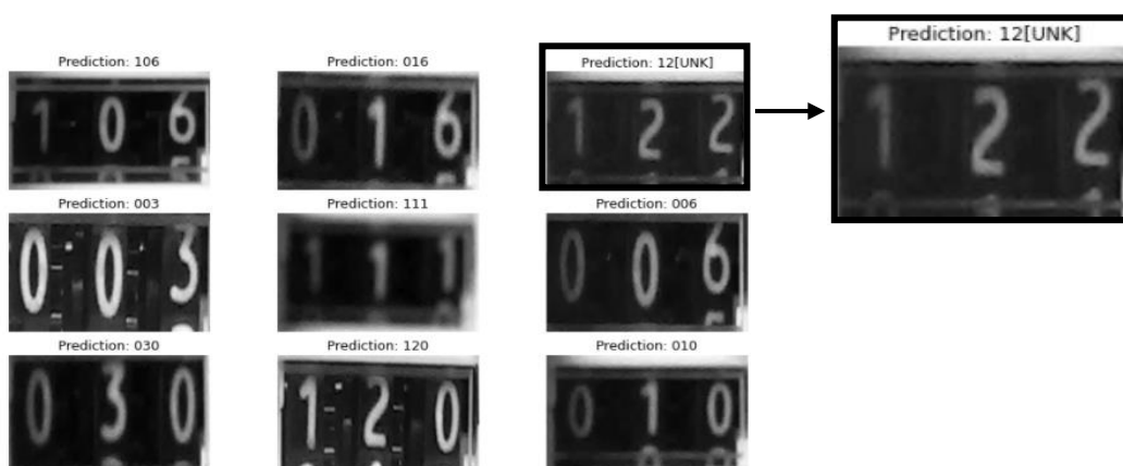
Figure 19 - Sample of the predicted text of the trained model, accompanied by the original images of the validation dataset.
