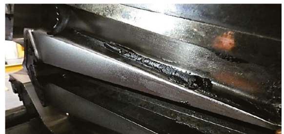
Fig. 13. Vulcanized rubber on the flow channel walls.
