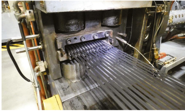
Fig. 2. Representation of a Cap strip line extruder head with cap ply strips being produced.
