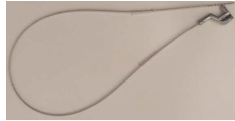
Fig. 1. Finished product – wire rope with end fitting.
