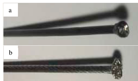
Fig. 3. (a) Hammered Coated and (b) Non-Coated Wires.
