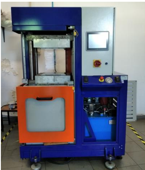
A 2 - Hot plates press and detail of the hot plates
