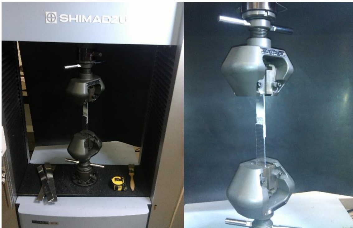
A 7 - SHIMADZU electro mechanical testing machine and specimen testing
