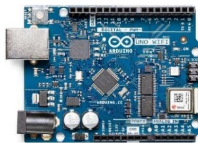
Figura 3.10 - Arduino Uno Wifi Rev2.
