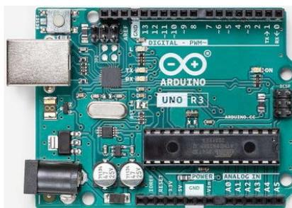
Figura 3.9 - Arduino Uno Rev3.
