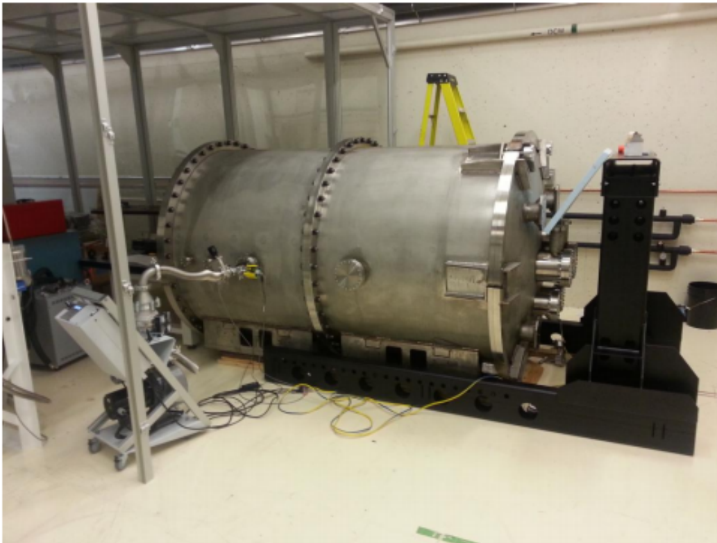
FIGURE 3.1: SPIRou cryostat at the National Research Council (NRC) Herzberg Astronomy and Astrophysics Research Centre. A cryostat is a device which keeps low cryogenic temperatures. From Moutou et al. [2015]
