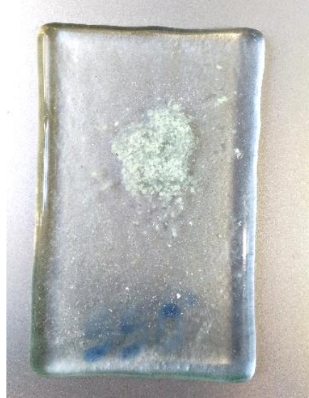
Figure 5-47. Fused Nemoto luminescent green frit on 3mm normal float glass at 850°. ©Parinaz Faghihi.
