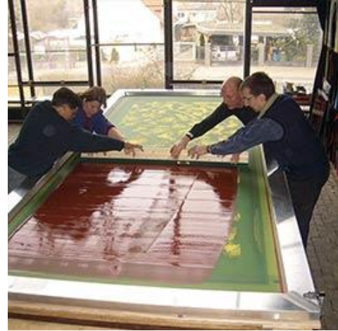
Figure 2-38. Squeegees color through large screens – Project for Portnoy Residence in Hillsborough, USA, Design by the cooperation of artists Janssen and Wood. ©2019 Derix Glasstudios.
