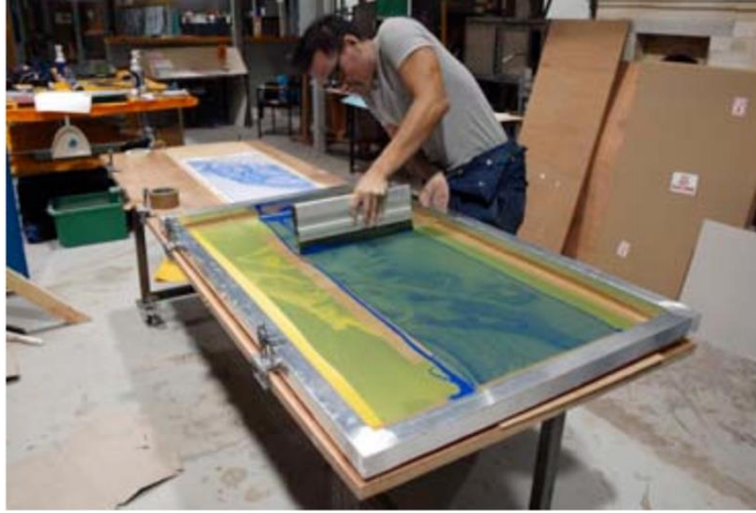
Figure 2-37. Jeffrey Sarmiento Screen printing enamels onto a long sheet of glass. ©Jeffrey Sarmiento
