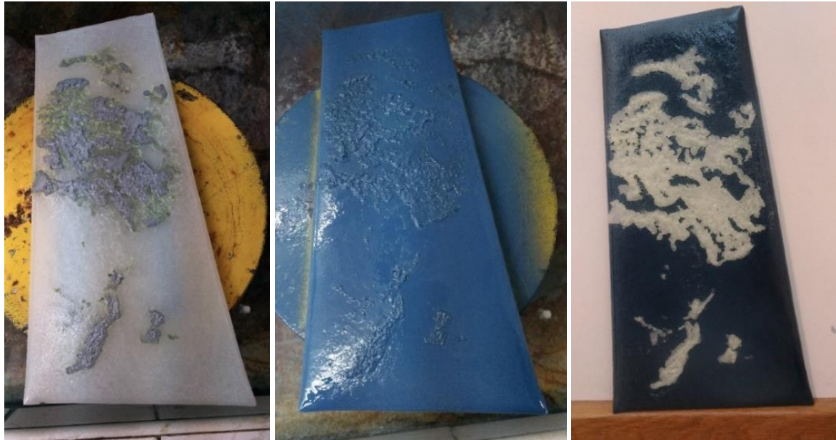
Figure 5-50. The process of making Sample 1. The luminescent parts are covered by liquid masking film, painted by airbrush, and fired in the kiln. ©Parinaz Faghihi (23.01.2018).
