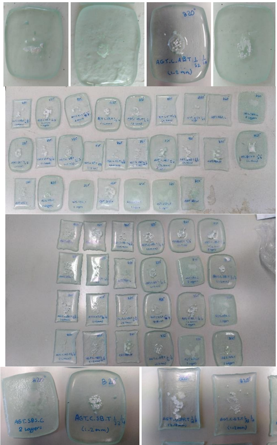
Figure 5-45. Result of fusing luminescent sand and stones of AGT™ company in 820 degrees and 850 degrees. ©Parinaz Faghihi.
