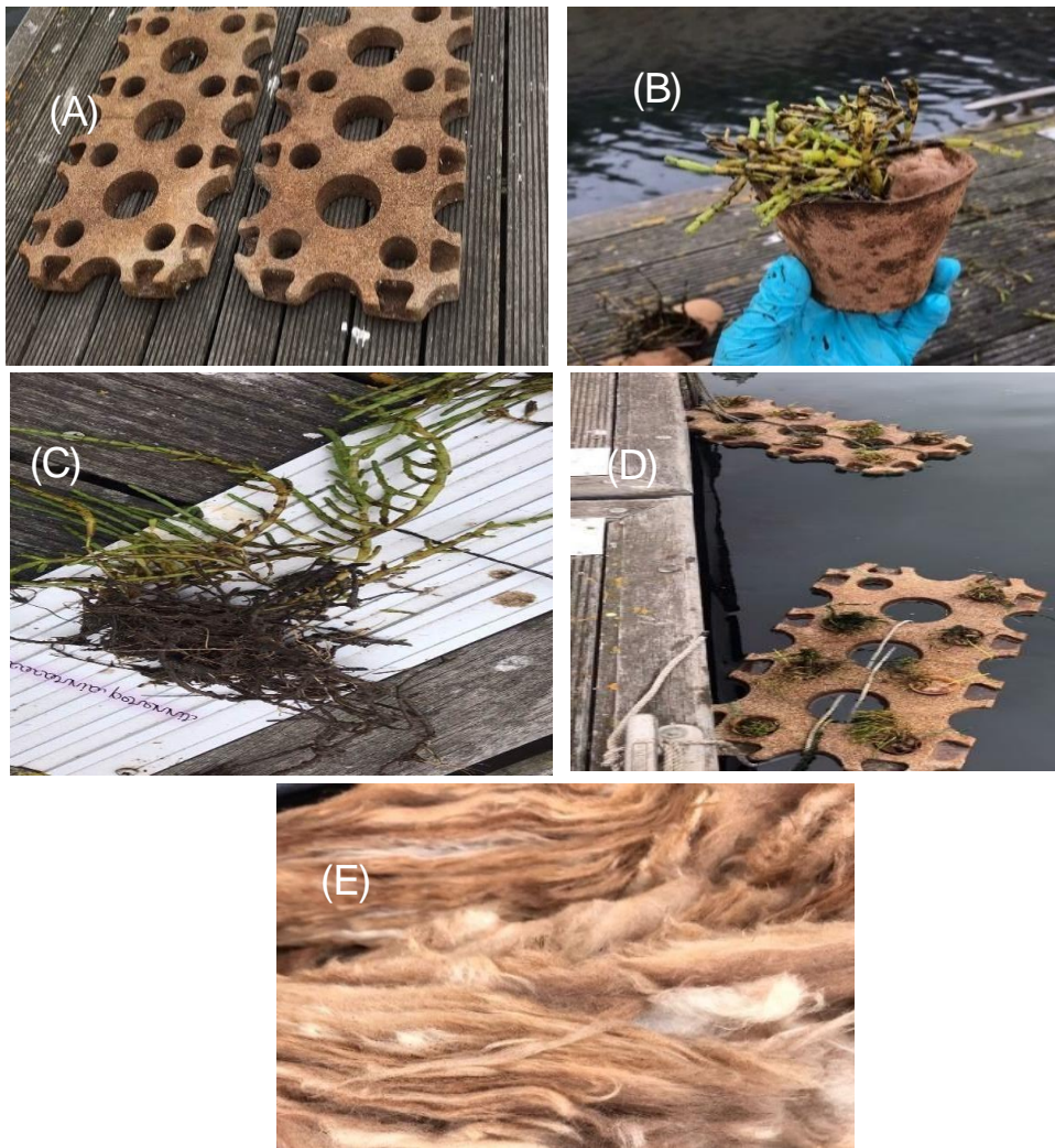
Figure 13: Floating Wetland Island at Porto de Leixões. (A) Module made of agglomerated cork (CORK FLOATING ISLAND®). (B) Sarcocornia perennis inside the vase. (C) Sarcocornia perennis . (D) System after assembling. (E) Rock blanket.
