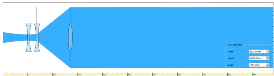
FIGURE 3.3: Simulation performed with the software GaussianBeam for the beam's vertical component.
