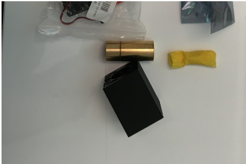
FIGURE 2.6: Cylindrical and parallelepiped-shaped pieces of aluminium that serve as heat sink for the laser diode.
