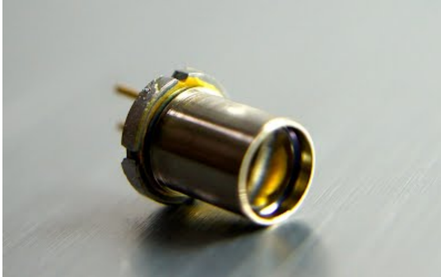
FIGURE 2.1: Nichia NUBM07E 465nm laser diode
