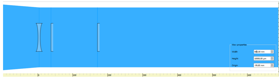
FIGURE 3.2: Simulation performed with the software GaussianBeam for the beam's horizontal component.
