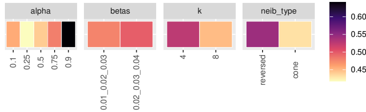
Figure 4.5: Percent rank obtained by each parameter setting, averaged over all experiments that used them in combination with each learning model and across data sets. Lower ranks indicate better performance
