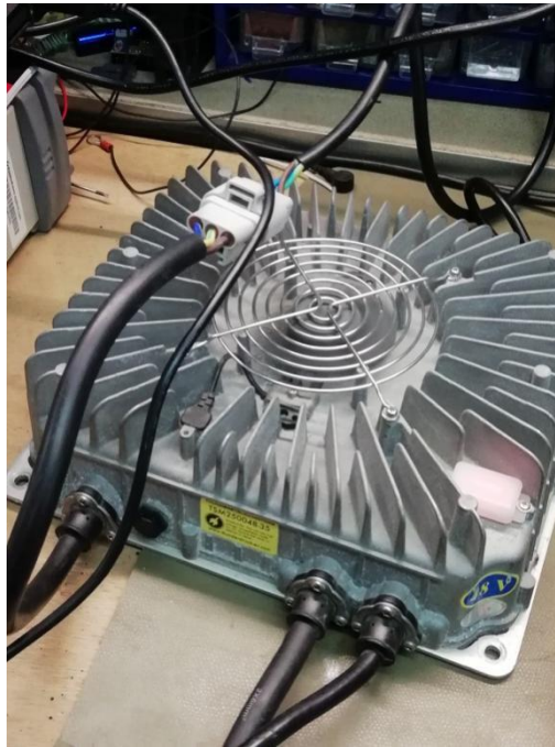
Figure 29 - Electrical battery charger
