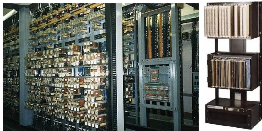
Figure 12 - Primary automated systems, Relay cabinet (adapted from [30]) (On the left) and MODICON 084 (adapted from [31]) (On the right)
