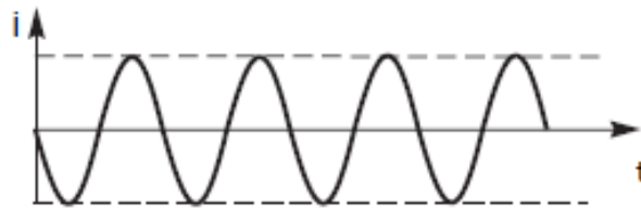
Figure 11- Symmetrical AC wave.
