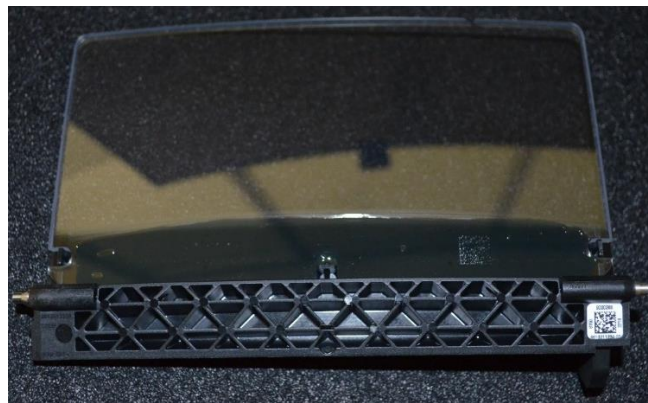
Figure 20 – Combiner Support (left) and Combiner (right) separated
