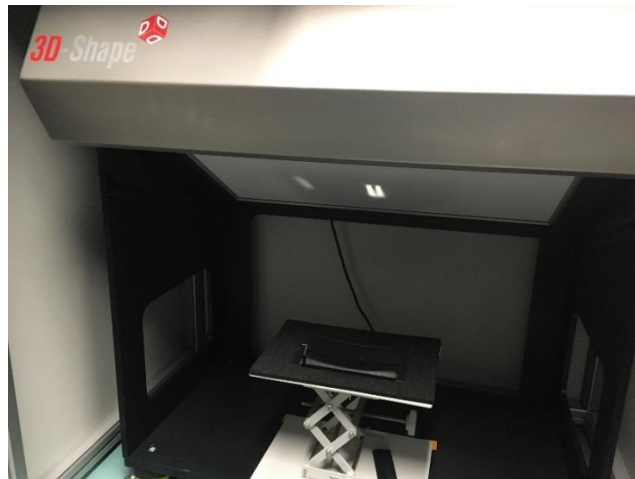
Figure 40 – 3D shape measuring setup
