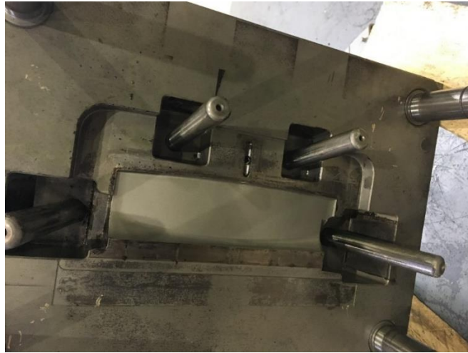
Figure 26 – Combiner Support injection mold
