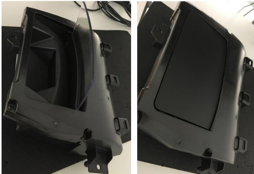
Figure 22 – Combiner Unit visible (left) and retracted (right) in the CHUD
