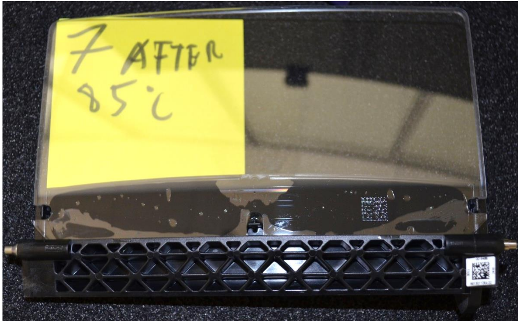
Figure 64 – Part number 7 after the thermal cycle
