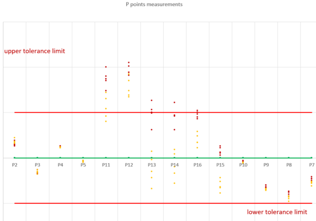
Figure 37 – P points (in mm) measurements after the oven 24 hours later in Yellow and in Red the measurements before the oven
