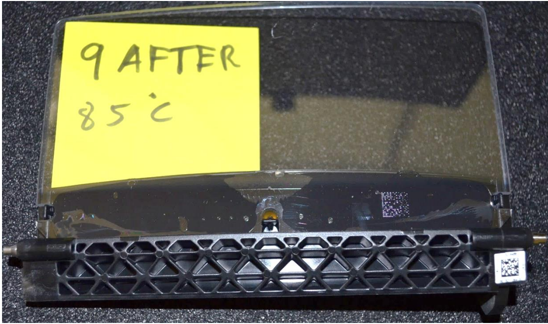
Figure 67 – Part number 9 after the thermal cycle
