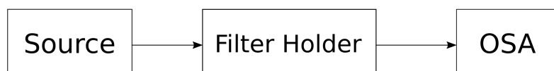
FIGURE 3.21: Schematic of the setup assembled for testing the filter and the filter holder.
